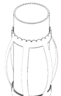
is claimed in the features of shape and/or configuration of the centraliser shown in solid line in the accompanying representations. The notches separating the circumferentially spaced teeth at the opposed ends of the centraliser body may vary in the number and dimensions.
