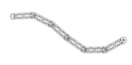
the accompanying representation. Any number of barriers may be interconnected end-to-end to form a composite barrier of varying shape and length.
