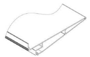
of the Shelving Wing Extrusion - The drip spike on the rear base of the Shelving Wing Extrusion.
