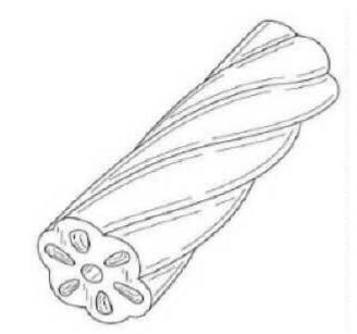
distinctiveness of the design lies in the features of shape and/or configuration depicted in the attached representations, including the following: a flower-shaped cross-section comprising six flower-shaped "petals" arranged radially around a central hole, each petal containing a seed-shaped hole and extending from the back to the front of the product as a twist along the product's length. The product is of indeterminate length.
