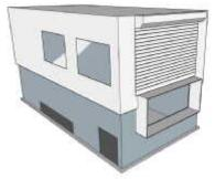
mounted to the outer body shell while the end of the roller door itself is attached to the upper part of the inner body shell - thus allowing the door to roll and unroll at the same rate as the body lift and keeping the inside of the motorhome body protected and insulated from outside elements and environment.
