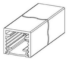
(57) Statement of Newness and Distinctiveness: The shape and configuration of a railing of constant cross section and indefinite length as depicted in the representations, wherein the break shown in the representations indicates the indefinite length of the railing.
